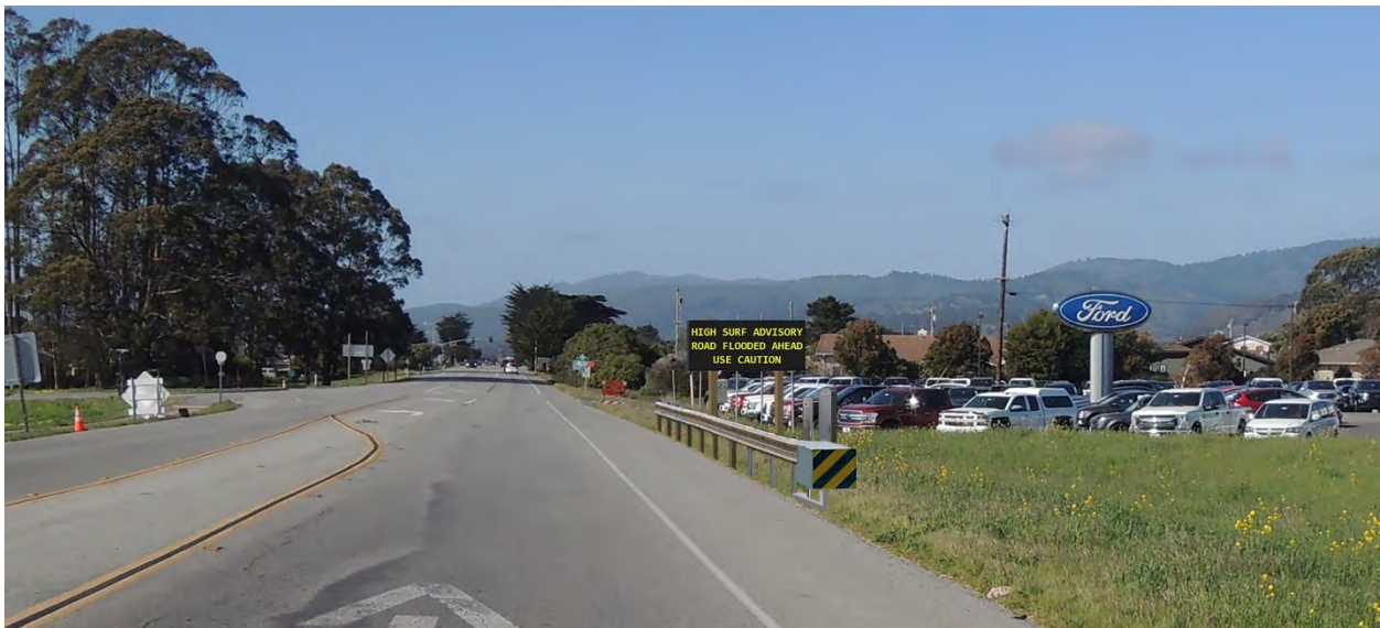
Figure 1-7 Visual Simulation of VMS (shown with message displayed) and MGS at Location 2
